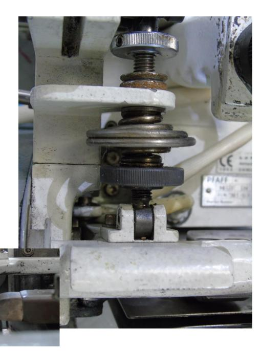
This screw controls the tension of the drive roller if this is to tight it produces drag that effect as it works as a potential
