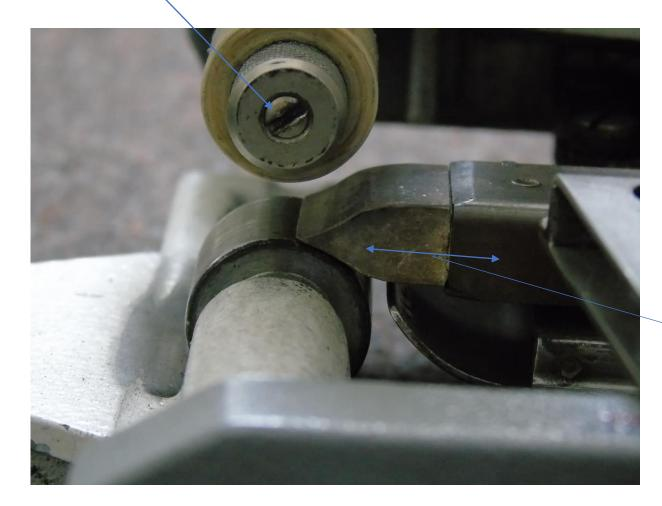
The wedge can move forward and back to allow for readjustment as it wears. To far forward and it will work as a brake. To far back and it will impact the bonding of the material. As the wedge is used it will require occasional cleaning and reshaping.
