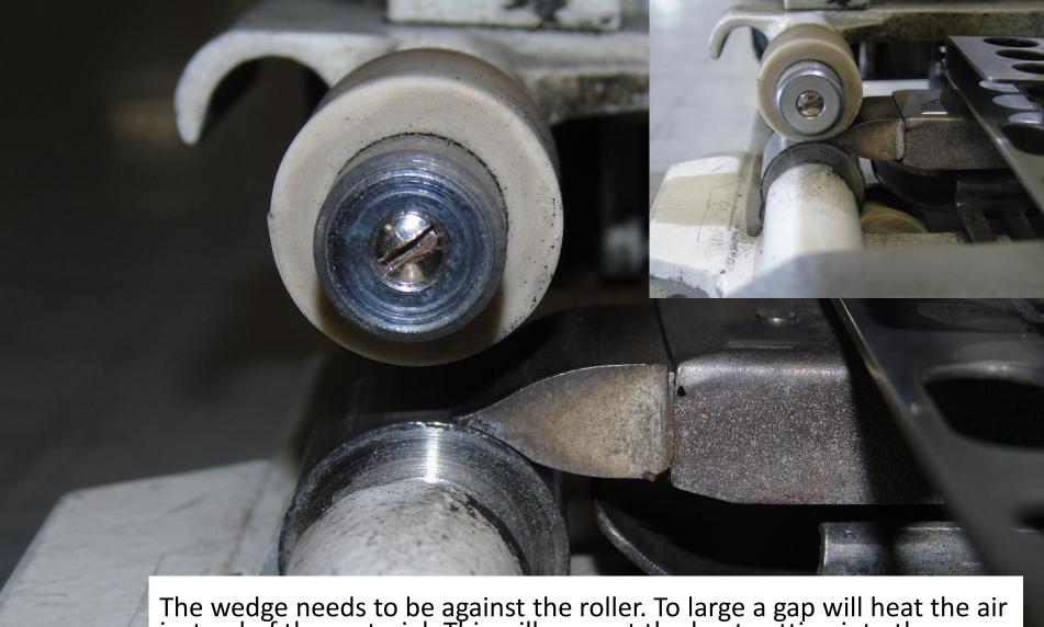
The wedge needs to be against the roller. To large a gap will heat the air instead of the material. This will prevent the heat getting into the material and stop the material being drawn across the wedge, disturbing the surface and helping with bonding the material.
