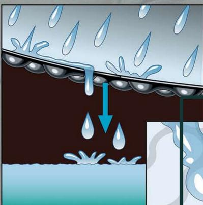
The addition of holes in the cover means that the VapourGuard<sup>TM</sup> material can help to harvest water, while also reducing evaporation.
