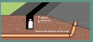
With the underlay and liner now installed the overflow pipe can be installed a by an experienced liner installer. A freeboard of 300mm is typically used, however local guidance on this issue may be required, as additional regulations may apply. Depending on design, location, and equipment available several different fall systems can be used.
