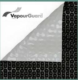
The light grey reflective surface reflects the suns heat away from the water, reducing the water temperature. Most bacteria grow rapidly in warm water and by reducing the water temperature the risk of bacteria growth is reduced. The black underside prevents light from penetrating through the cover, photosynthesis does not occur, thus starving algae of any nutrients to grow, eliminating algae growth.
