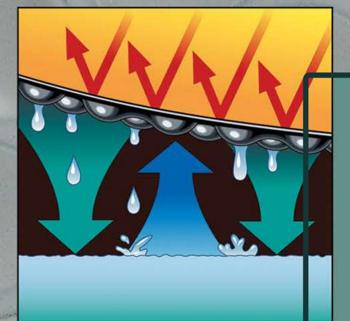
VapourGuard™ material provides evaporation control, algae inhibition, debris reduction and temperature regulation. The material can be applied in modular sections or as a complete covering membrane to the surface of the water. With the addition of small holes during the fabrication process the cover can also be used for rain water harvesting.
